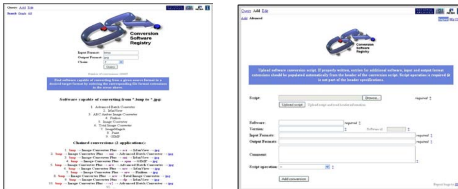
Figure 2. Left: The CSR web interface showing a conversion query to find the shortest conversion path between the two formats entered. The single and multiple path conversions are listed alphabetically. Right: A form for inserting software information.
