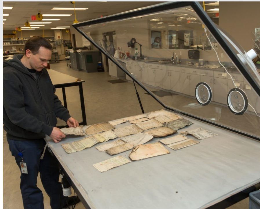
A preservation technician places documents from an Official Military Personnel File (OMPF) damaged in the 1973 fire in a humidification dome.
