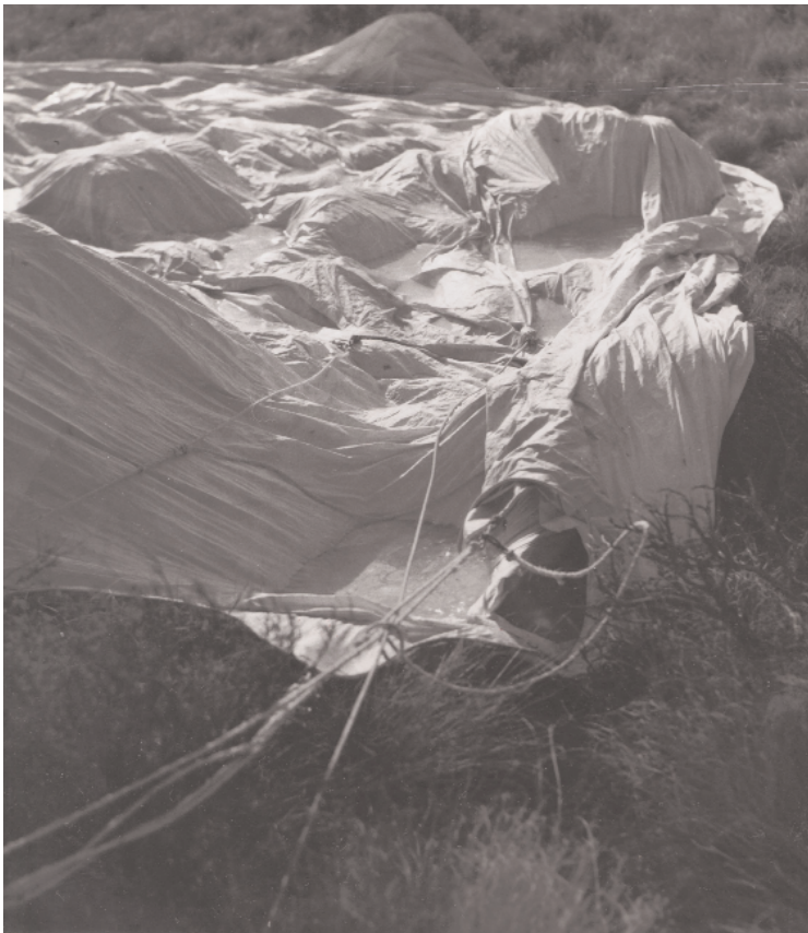
Above left: Prossor Balloon—Section of bag, as found. (Note ice that has formed.) Reproduced at the National Archives and Records Administration—Pacific Alaska Region (Seattle)
