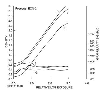
These curves depict the Diffuse RMS Granularity as a function of exposure. The sensitometric curves are shown so that the granularity as a function of density can be estimated. Because the granularity of the intermediate film is lower than the granularity of any original negative, the intermediate film will add little or no granularity to the final print.
