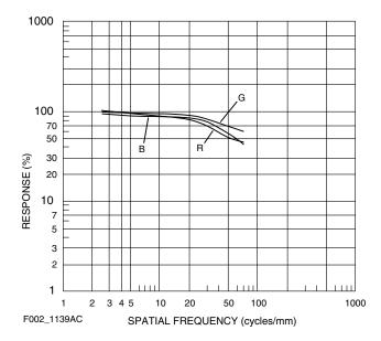
These curves depict the response of the film to image detail, which can be mathematically expressed as a series of frequencies. The ability of the film to reproduce frequencies at or near 100% over a long range means that the film will copy the original negative with little or no loss in sharpness.
