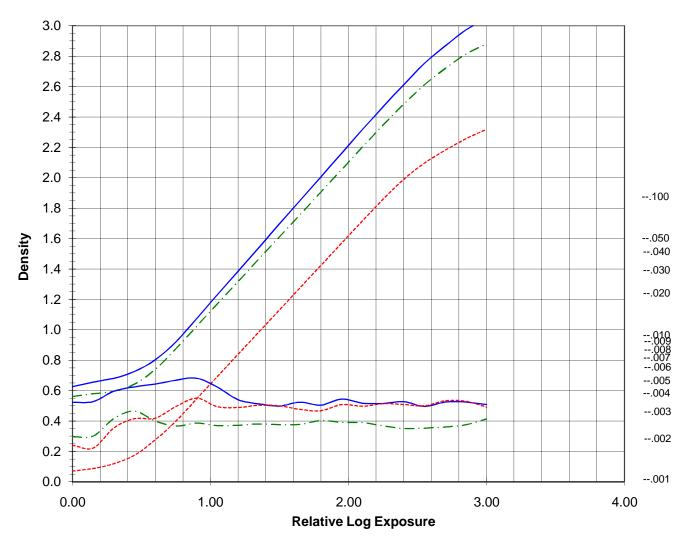
Granularity SIGMA D x 1000
