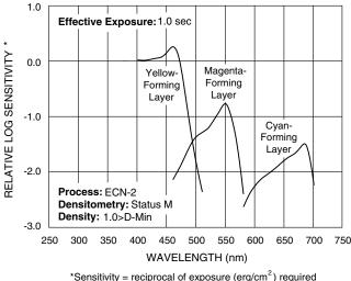
\*Sensitivity = reciprocal of exposure (erg/cm²) required to produce specified density
