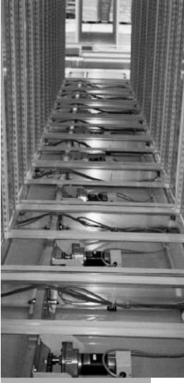
The carriages feature a welded aluminum uniframe construction, which provides a high strength-to-weight ratio; prevents binding, racking, and misalignment; and eliminates the need for fasteners that can loosen or break.
