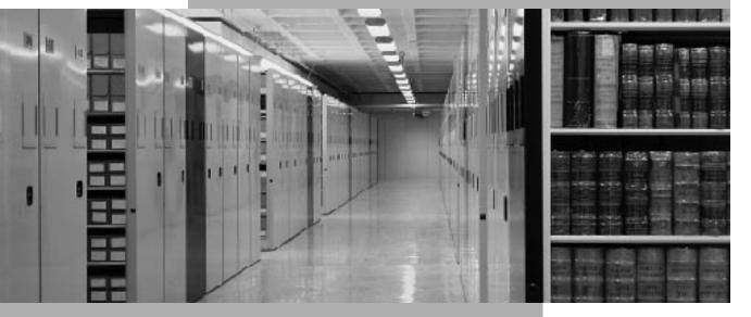
The system compacts almost 2 million cubic feet of storage capacity into an area of 691,572 square feet. The 2,000 carriages roll on more than 80,000 feet (over 15 miles) of rail recessed in the concrete floor.
