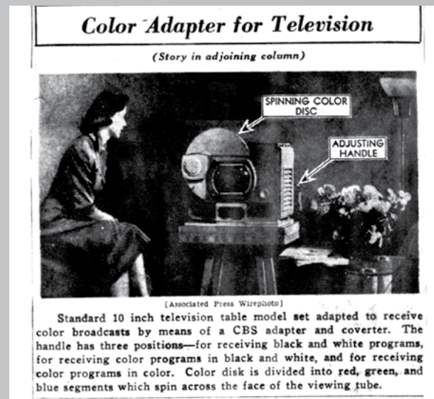
A newspaper article illustrates the new CBS television model of the late 1940s that could display color images using a rotating disc with color segments that spun quickly in front of the viewing tube.
