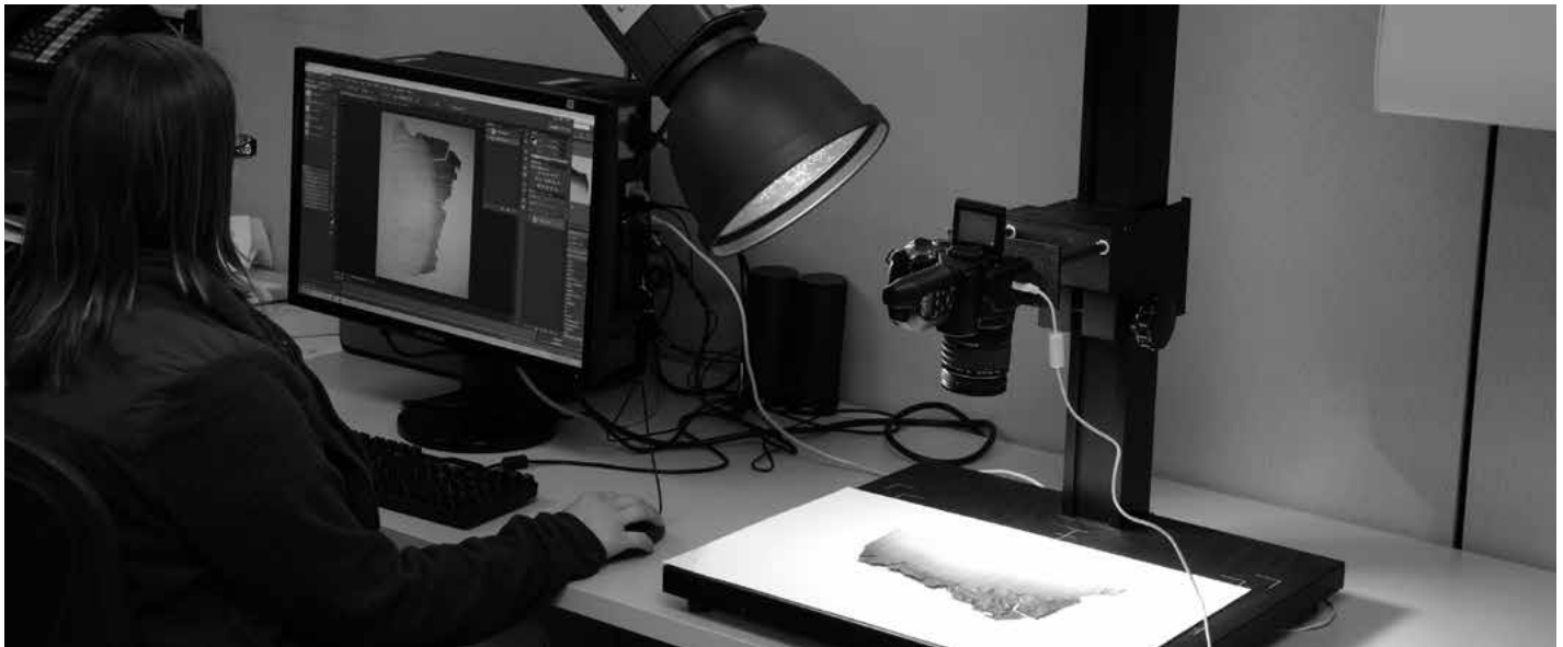
Preservation technician Meghan Krato uses an infrared camera and computer software to recover lost information on a burned record.
